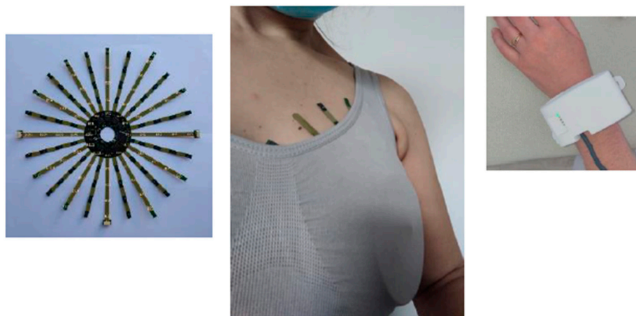
Figure 1. Photograph of the PHI-BRA sensor centered around the nipple and held in place by a sport bra. The data acquisition unit is placed on the participant's wrist.
